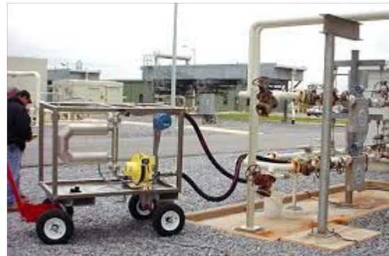
A portable calibration rig in use at an airport
